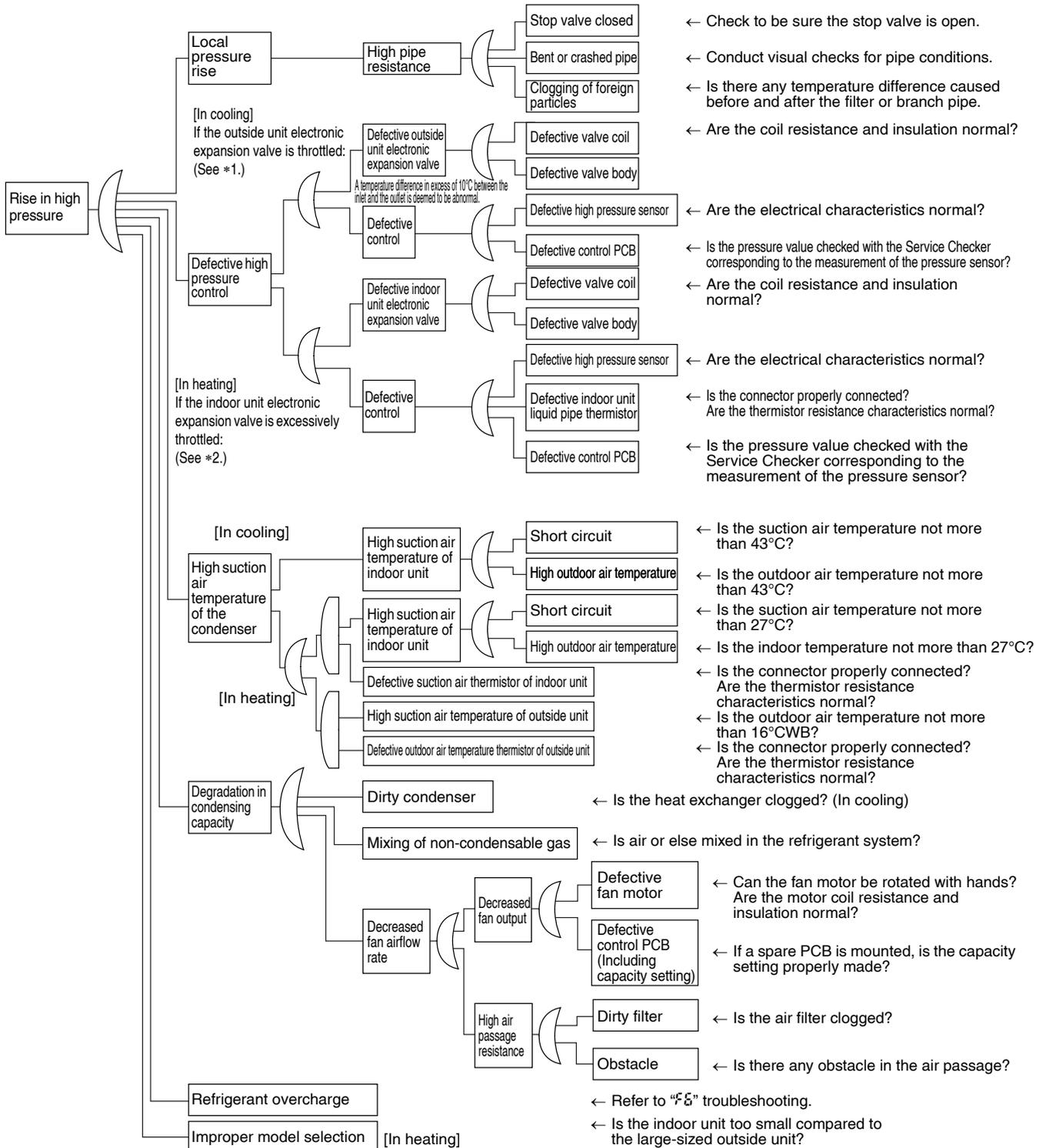
\*1: In cooling, it is normal if the outside unit electronic expansion valve is fully open.
