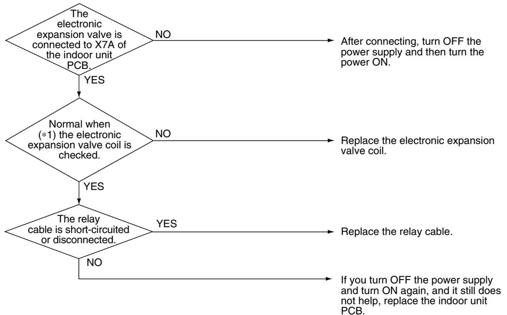
**i Note:** \*1: Make measurement of resistance between the connector pins, and then make sure the resistance falls in the range of 40 to 50Ω.
