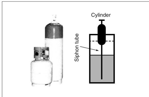
Refrigerant can be charged in liquid state with cylinder in upright position.
