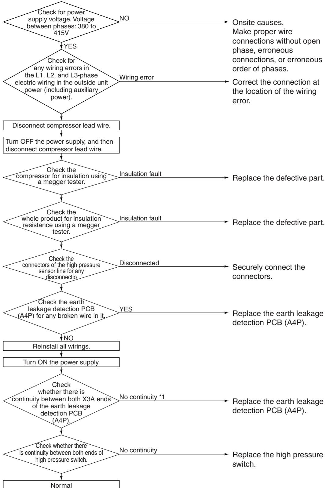
It is supposed that ground leakage occurs due to temporary liquid back or accumulation of refrigerant. This phenomenon can occur when power fails while in operation or is cut off for an extended period of time.
