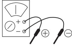
\* Preparing a tester in the analog system is recommended. A tester in the digital system with diode check function will be usable.
