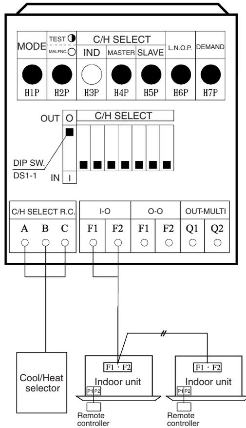
**(3) Set Cool / Heat for more than Single Outside Unit System Simultaneously in Accordance with Unified Master Outside Unit by Indoor Unit Remote Controller**
