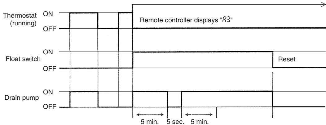
During heating operation, if the float switch is not reset even after the 5 minutes operation, 5 seconds stop, 5 minutes operation cycle ends, operation continues until the switch is reset.
