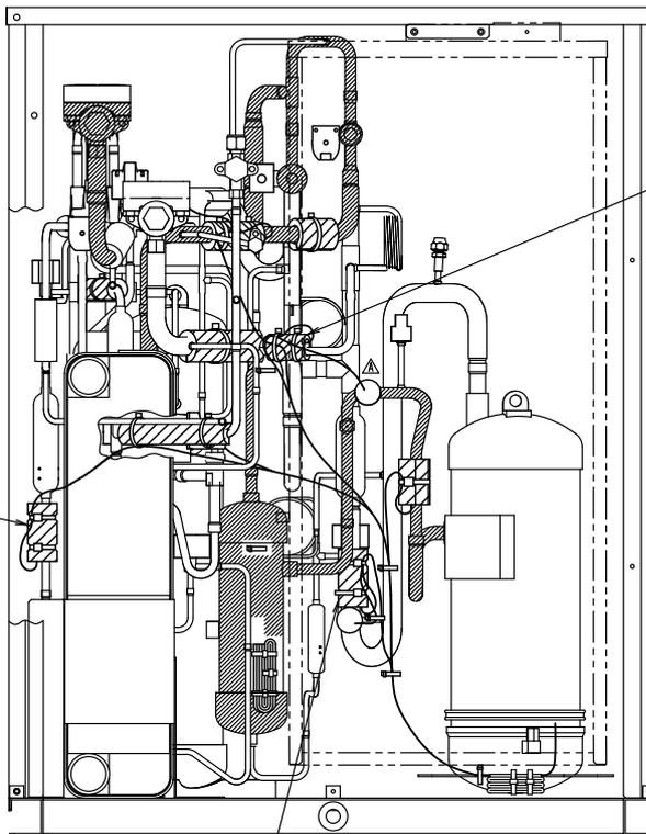
Subcooling heat exchanger outlet pipe thermistor (R5T)
