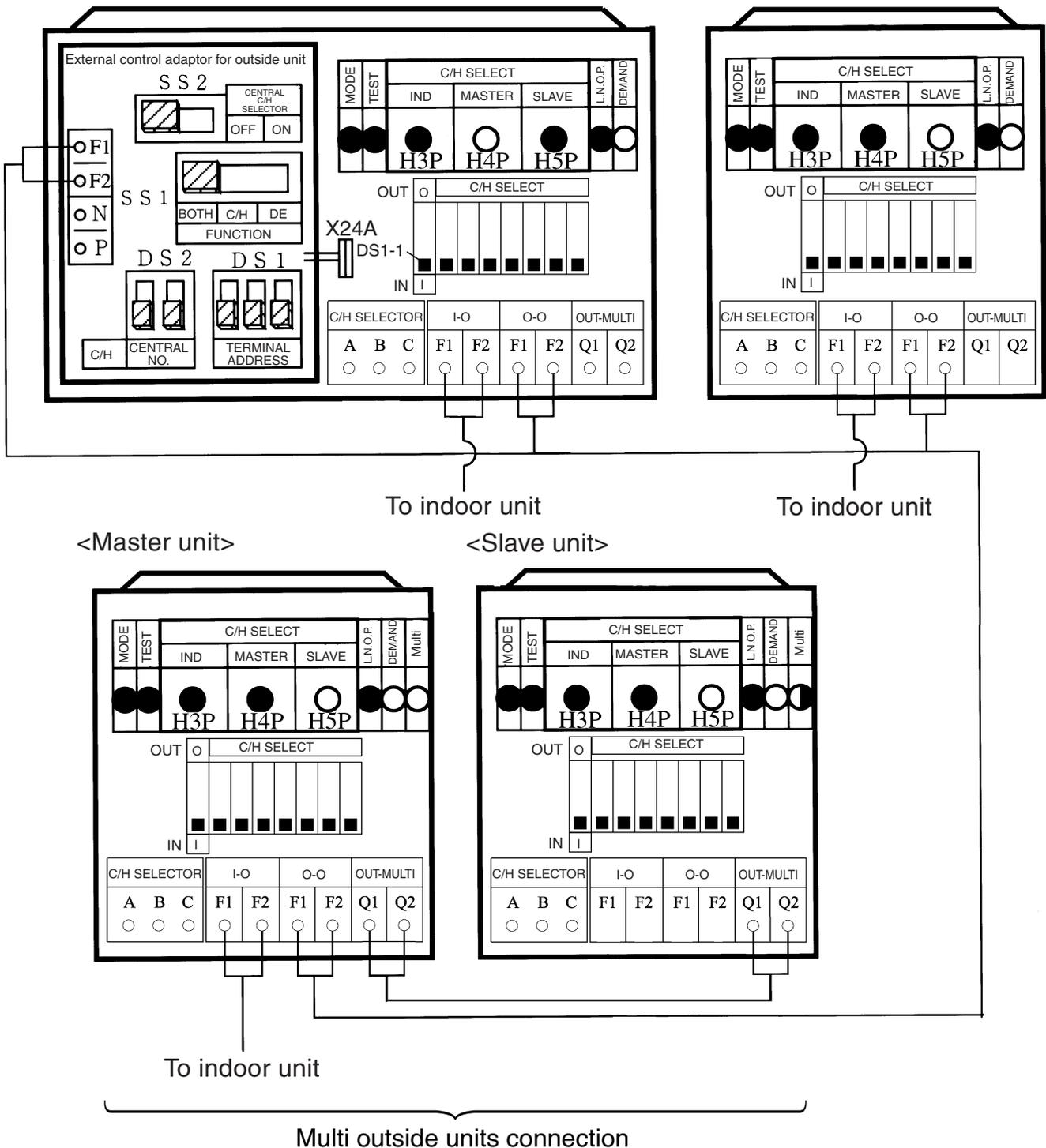
**(4) Set Cool/Heat for more than Single Outside Unit System Simultaneously in Accordance with Unified Master Outside Unit by Cool / Heat Selector**
