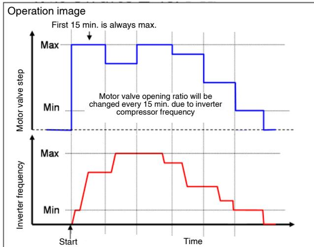
Depending on the capacity step of the compressor, the position of the water flow control valve is adjusted in maximum 13 steps.
