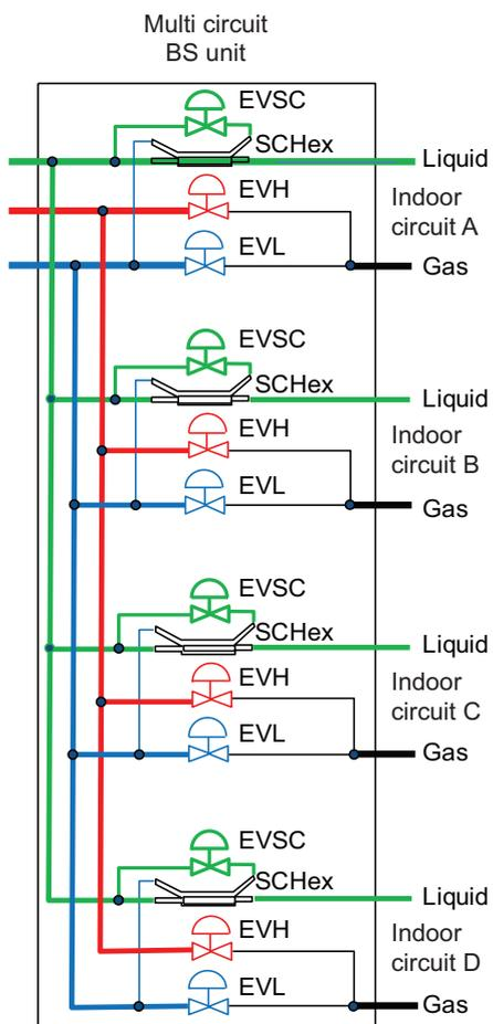
Each indoor circuit offers the possibility to connect the indoor gas pipe:
