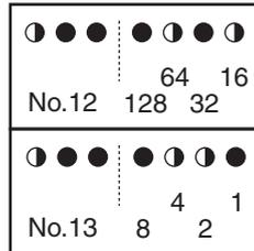
In (Example 2) the address for No. 12 is 0101, the address for No. 13 is 0110, and the combination of the 2 is 01010110 (binary number), which translates to  $64 + 16 + 4 + 2 = 86$  (base 10 number). In other words, the number of terminal block is 86.
