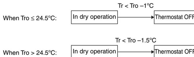
Furthermore, while in dry operation mode, fans operate at "L" tap, stops for a period of 6 minutes while the thermostat is OFF, and then return to operation at "L" tap. (This control prevents a rise in indoor temperature while in thermostat OFF mode.)
