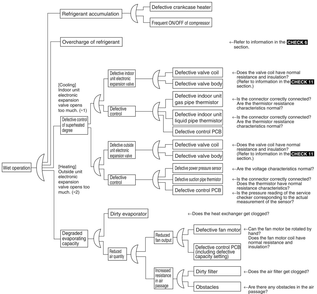
\*1: "Superheated degree control" in cooling is exercised with the indoor unit electronic expansion valve.
