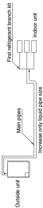
Note 2. Allowable length after the first refrigerant branch kit to indoor units is 40m or less, however it can be extended up to 90m if all the following conditions are satisfied. (In case of "Branch with REFNET joint")
