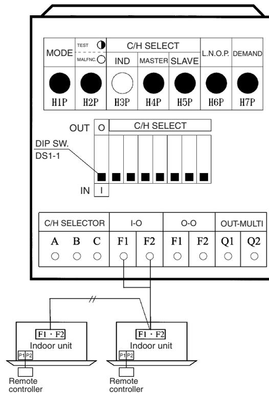
**(2) Set Cool/Heat Separately for Each Outside Unit System by Cool / Heat Selector**
