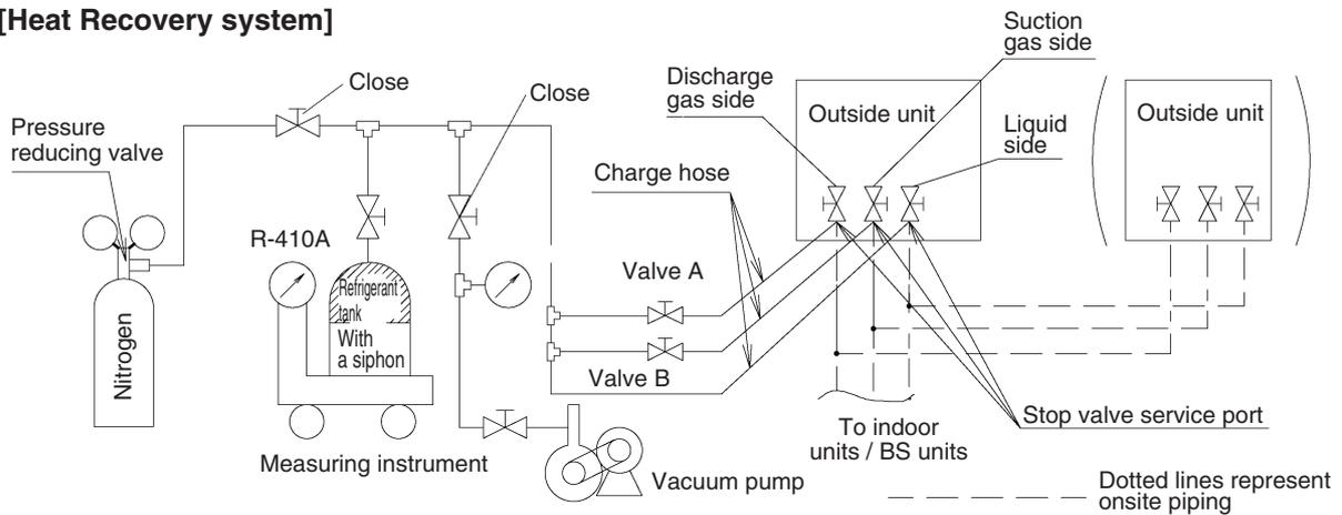
**Additional refrigerant charge procedure (2)-by Additional refrigerant charge operation**
