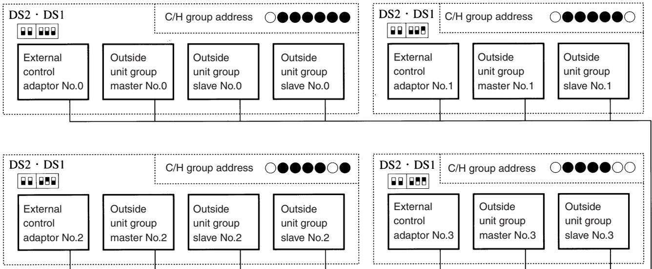
**Address setting for (3) and (4) (Set lower 5 digits with binary number.) [No.0 to No.31]**
